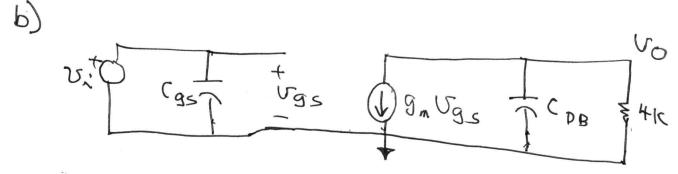
Summing currents at output node with  $G_L = \frac{1}{4k}$   $V_O(SC_{OB} + G_L) + g_m V_i = 0$
